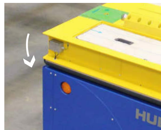
Platform truck for transporting the tail unit in a painting plant with platform lift
