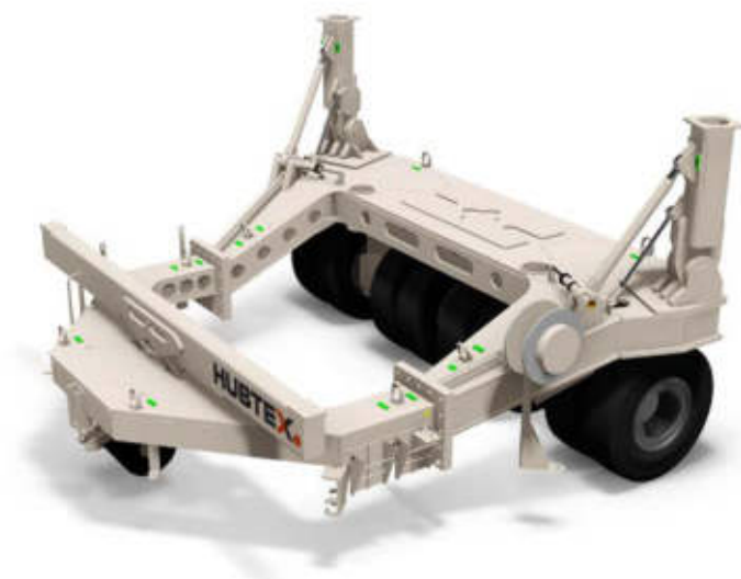
The FTT is docked and then the aircraft is lifted, transported and repositioned.
