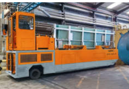
GTR 330 E unloading/ loading an autoclave in a laminating line
