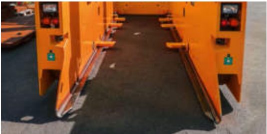
GTR with special device to transport glass stillages with fork pockets
