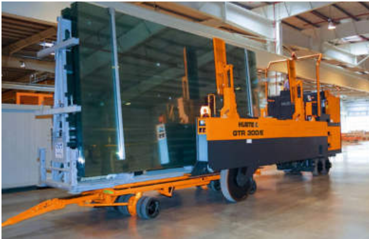
GTR unloading stillage from trolley
