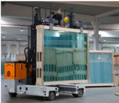
M 90 handling glass packs in end caps
