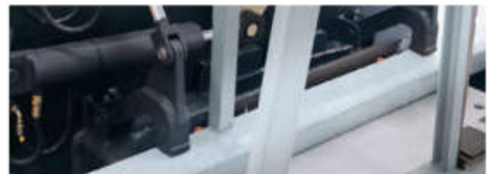
Glass securing device adjustable to different glass pack heights and widths
