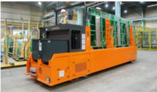
GTR 330 E for indoor transport of L-stillages with 33 tons of glass
